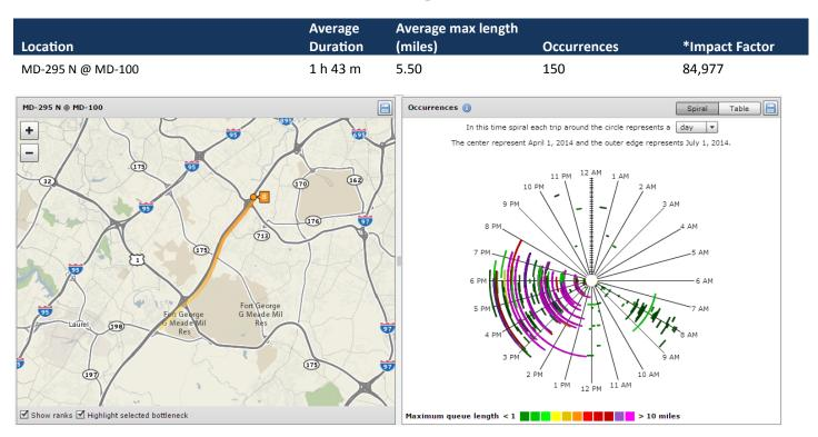
**Notes:** Recurring afternoon congestion. Level of Service "F" from 4:00 to 5:00pm. A primary cause appeared to be the discharge of traffic from NSA / Ft. Meade onto northbound MD 295 via the Connector Rd. Weaving and merging at the MD 32 interchange also contributed to the congestion **Source:** Skycomp Report
