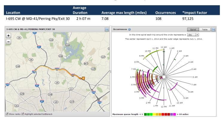
**Notes:** Congestion was most severe between I-83 and Providence Rd. Factors contributing to this long standing and extended congested zone: merging and weaving associated with traffic at each interchange and a lane drop (to 3 lanes) at MD-45/York Rd **Source:** Skycomp Report
