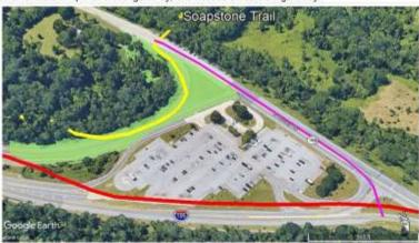
Proposed Patapsco Park Gateway where a parking lot is now located at the unfinished end of I-195 at Rolling Road. Patapsco Park now occupies the top area (Scepatione Trail), and would be expended into the green shaded area currently part of I-195, with its southbound roadway shifted to the red line next to the northbound roadway.
