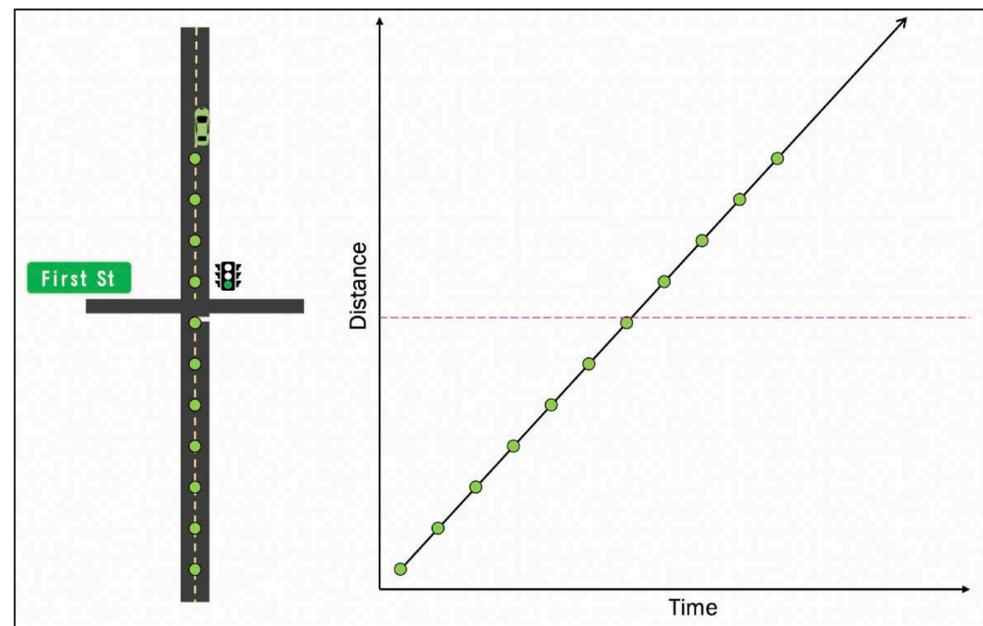
Figure 1. Trajectory Data and Time Space Diagram Example
