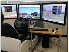
Two full-size driving simulators and a bicycle simulator at Morgan State's Safety and Behavioral Analysis Center allow us to research driver behavior and connected and autonomous vehicles.
