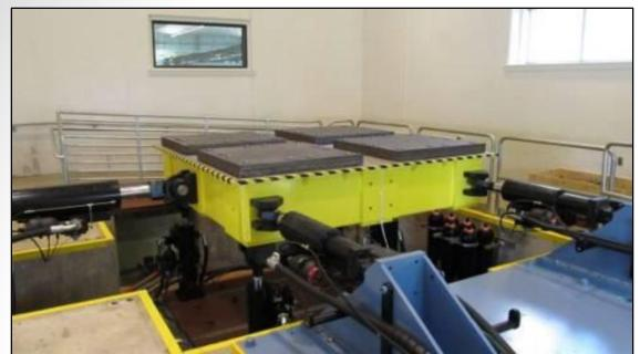
Morgan's structures and materials lab includes a shake table that goes up to 8.0 on the Richter scale.
